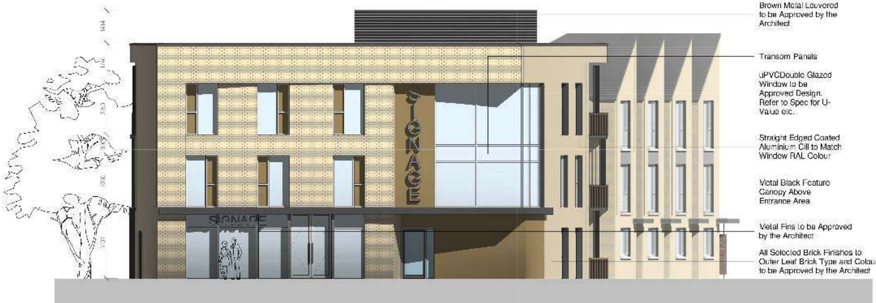
2 Block F - North Elevation 1:100
